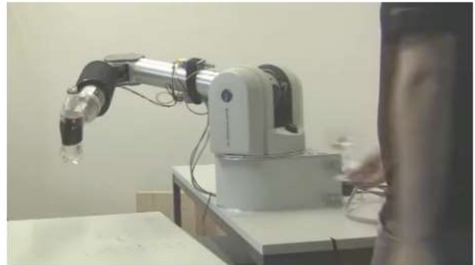
Too compliant: Liquid spills from glass
