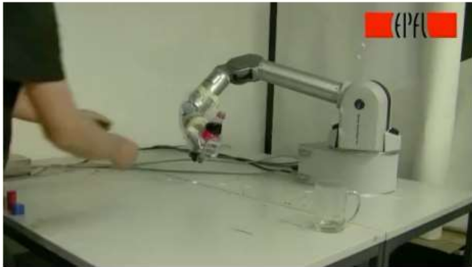
Too stiff: Liquid spills from jerking
